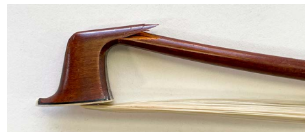
This is what can happen when a bow is tightened too much.
