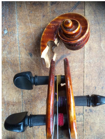
This damage could have been prevented if the pegs had been working properly.
